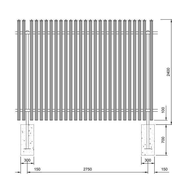
TYPICAL PALISADE FENCE ELEVATION
